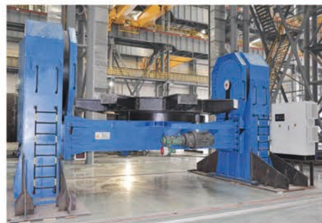
100吨焊接变位机 Welding positioner with capacity of 100 tons
