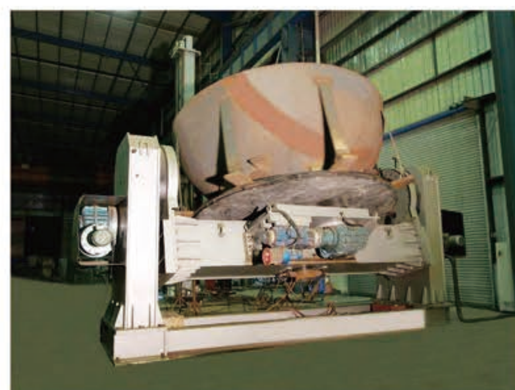
60吨焊接变位机 Welding positioner with capacity of 60 tons
